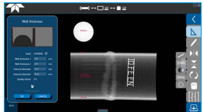
Wall thickness measurement
