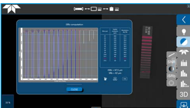
iSRb calculation and automatic IQI recognition
