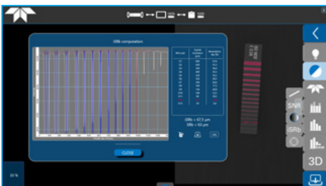
iSRb calculation and automatic IQI recognition
