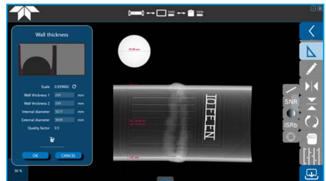
Wall thickness measurement
